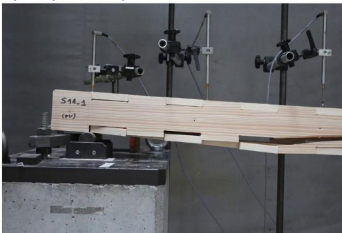
Shear failure in the connection
