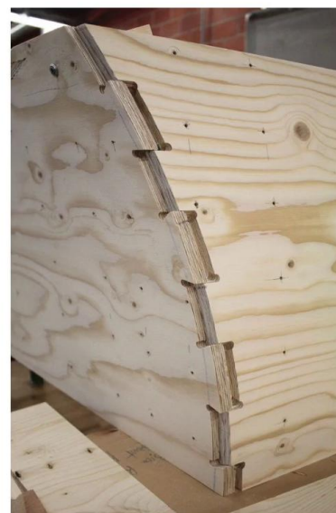
Dovetail Joints fit precisely
