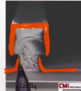
Cross section of sputtered Al on double layer lift-off resist. Large metal sidewall coverage under the T shaped resist. No real shadow effect.
