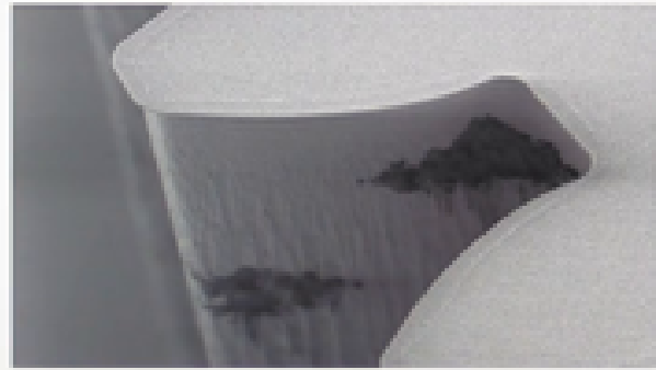
Lack of passivation: formation of local lateral holes on sidewalls
