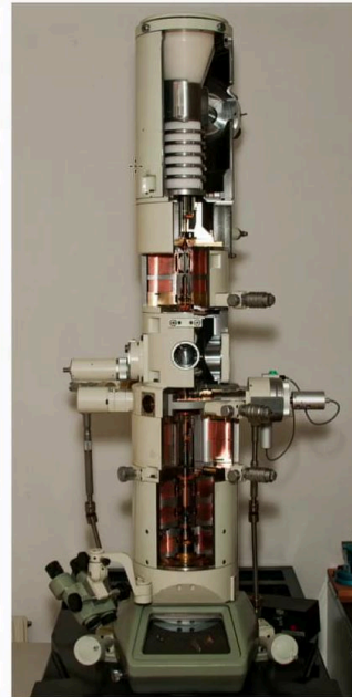
A typical TEM: Jeol 200cx Transmission Electron Microscopy
