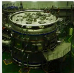
KSTAR- Daejeon 2007 Nb 3 Sn, He forced flow, 8T
